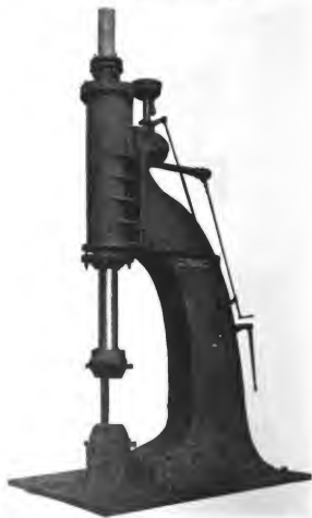
Fig. 9911. 2,000-lb. Single Frame Steam Hammer. William Sellers & Co., Inc.
